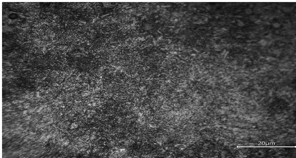
Figure 4.11. Optical Micrograph Image of 450oC Tempered Specimen Shown Under Magnification of X400
