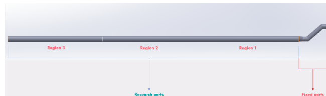
Figure 8: Racing exhaust designed from the assembly of several components made. The head exhaust section is used as fixed parts or fixed variables, and the research parts section, which consists of regions 1, 2 and 3 are independent variables.
