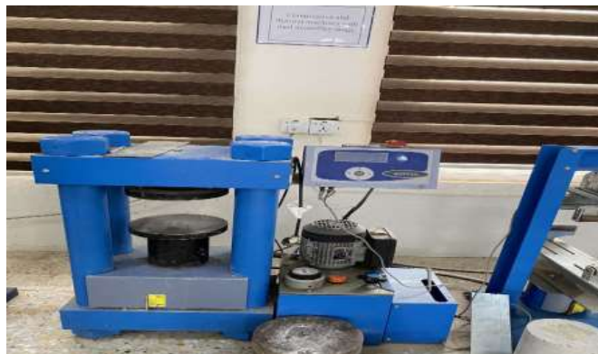
Figure 2: Testing the compressive strength of concrete cubes, Duhok Polytechnic University (2021).
