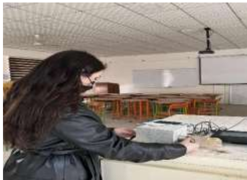
Figure 4: Testing the sound waves passing through concrete. Taken by the researcher 2021.
