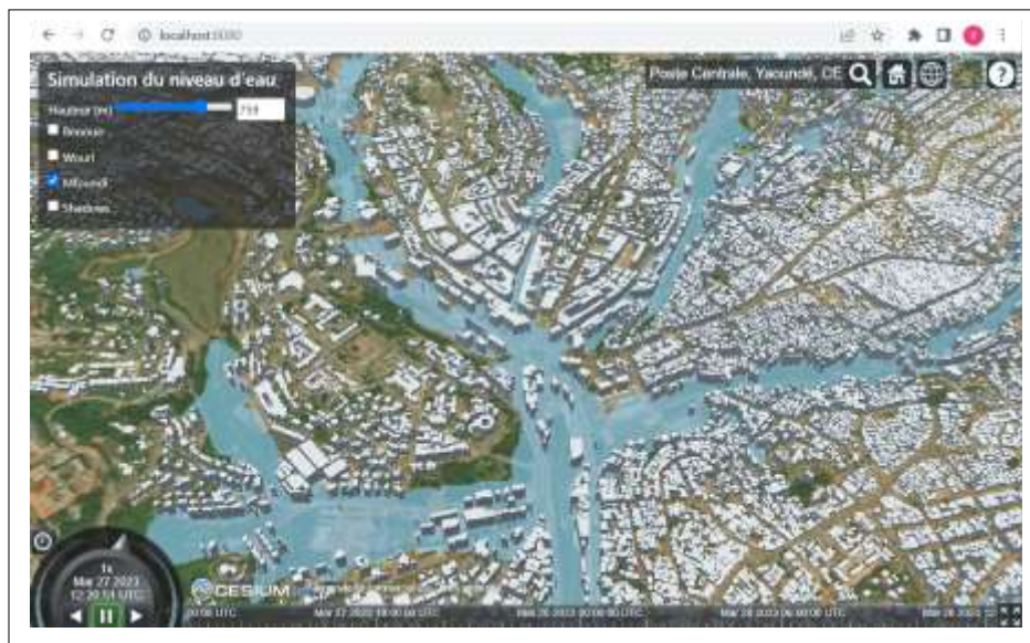
Figure 1. Simulation and visualisation of a flood at the Yaoundé central post office
