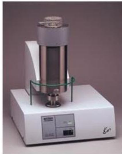
Fig. 1. Differential Thermal Analysis (DTA) Instrument
