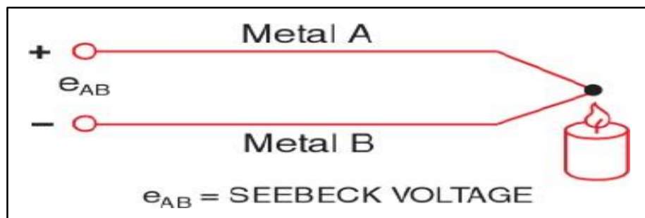
Fig. 2. The Seebeck Voltage Arising Due to Temperature Changes in a Thermocouple
