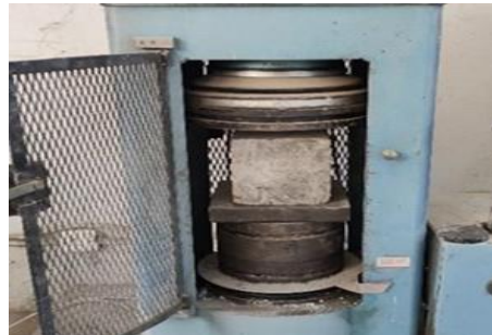
FIGURE3. Compressive strength test
