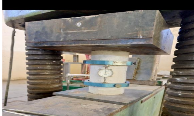
FIGURE8. Modulus of Elasticity Test
