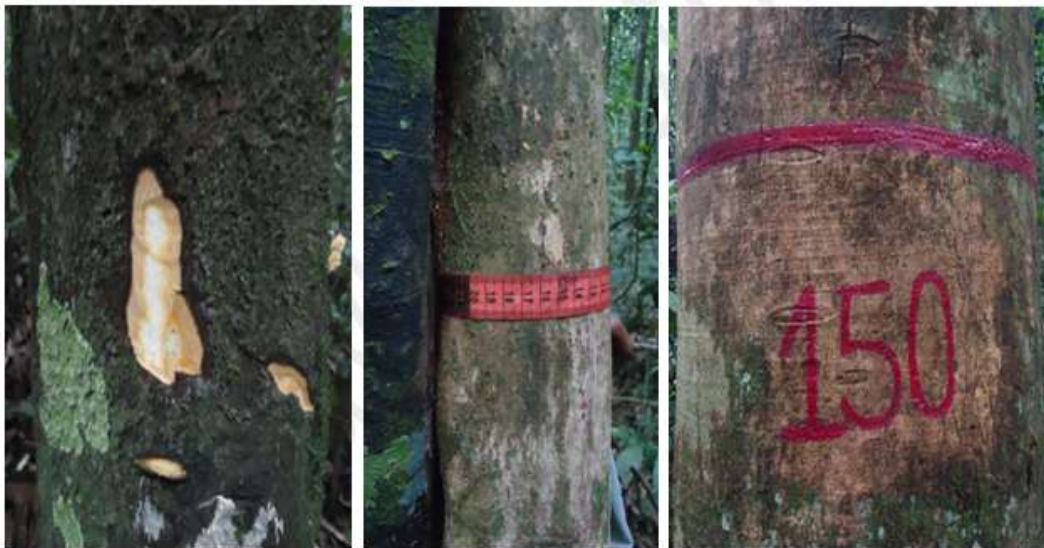
Photo 1 – Bark notch, dhp measurement and tree numbering and paint line (from left to right)
