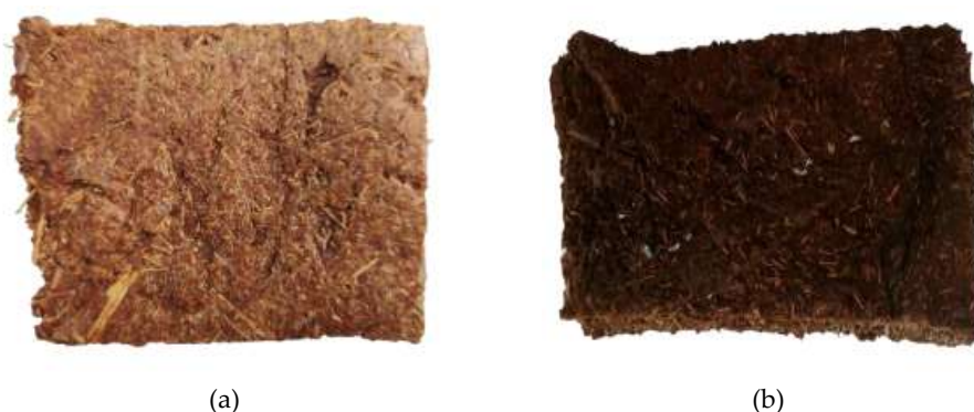
Figure 5: Biodegradable foam without chitosan (a) and with the addition of 10% chitosan (b)
